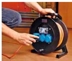
2 Mobiler FI-Schutz (RCD)
